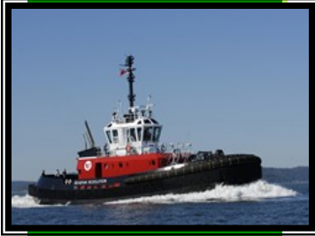
Seaspan's new tug the "Seaspan Resolution" With 82 tonnes of bollard pull, the tug entered service in July
